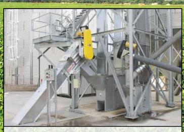
V-Bracing for Conveyor Access to Elevator Boot
