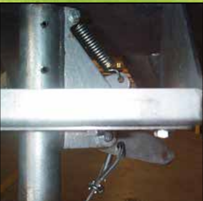
Spring tensioned latch mechanism.
