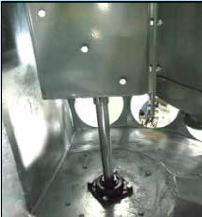
Swing spout rotates on a solid shaft with a flanged block bearing.
