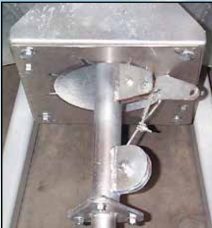
Positive locking index plate located under the distributor for protection from dust and weather.
