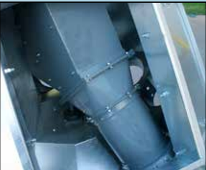
No tools required to open door for cleaning and maintenance. All internal parts can be disassembled and removed through the opening.
