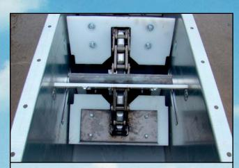
Each UHMW paddle bolts onto a large, formed steel backer plate that is welded onto the chain.
