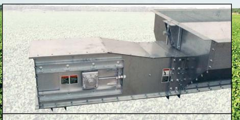
Screw take-up assembly on tail section and outboard mounted flange bearings with shaft seals.
