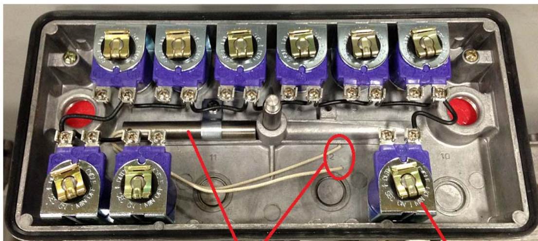
Goyen Multi Valve Enclosure w/ RCA3D2 Pilot Solenoid Valves (Cover removed for photo)
