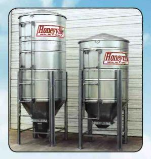
HONEYVILLE Economy Bins have a full 51" top opening for filling of bin with a hinged galvanized spun cover. These bins have a 52° center draw hopper and will handle free-flowing feeds such as hog or low fat poultry feeds and pelleted products.
