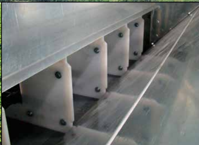
Smooth, self-cleaning slopes inside the pit hopper minimize clean-up.
