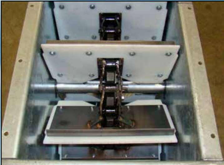
UHMW paddles bolt onto a large, formed steel backer plate that is welded onto the chain with secondary diagonal braces.
