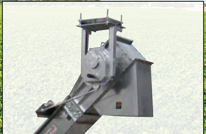
Head section 10 Ga. Galvanized steel with Class II Torque-Arm Type Gear and overhead motor mount.
