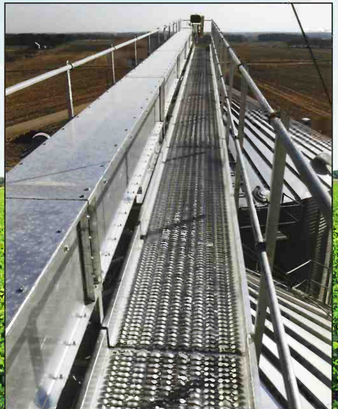
46" wide conveyor support: 22" for conveyor and 24" for galvanized grip surface walkway - 42" tall with handrail
