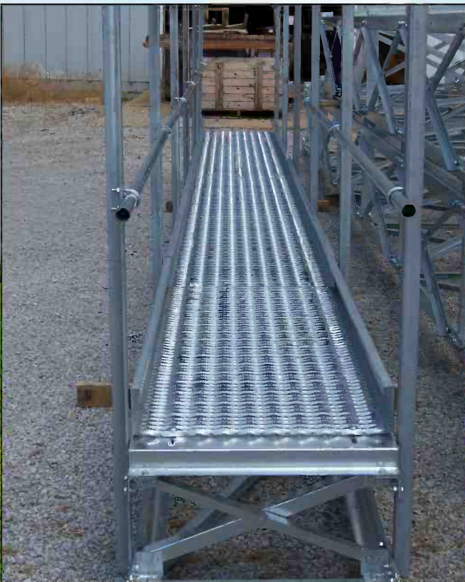
24" wide bridged manwalk: galvanized grip surface walkway, 42" tall handrail, 59" O.A. height
