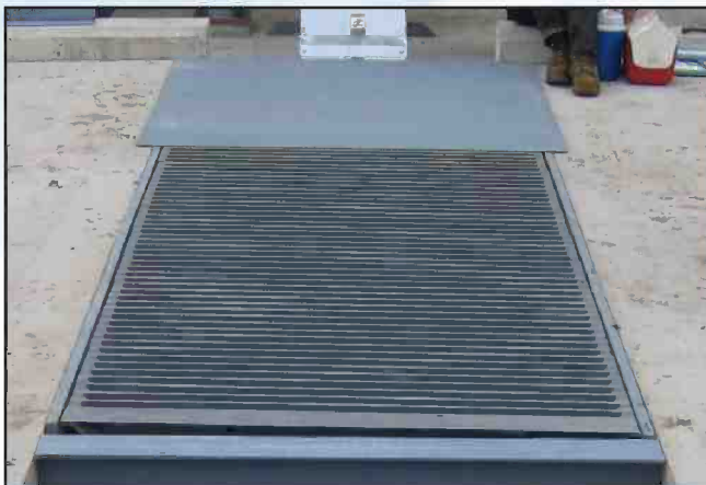
Drive-over pit hopper with bar grate provided in 12" wide lift-out sections for easy access
