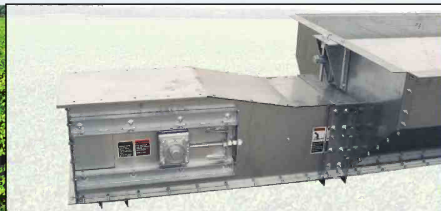
Screw take-up assembly on tail section and outboard mounted flange bearings with shaft seals
