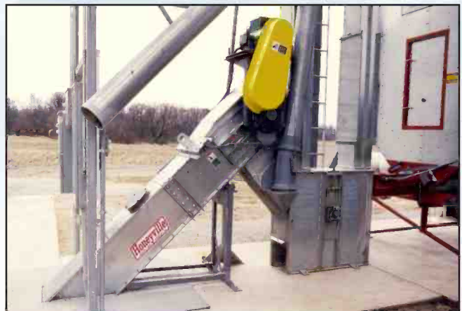
Typical application: Incline Drag Conveyor in a pit, feeding an elevator boot above grade
