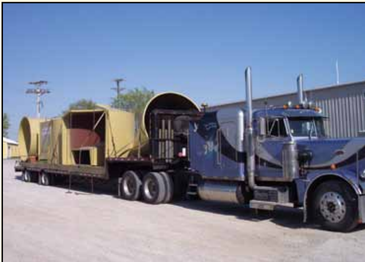
Larger diameter cyclones can be split vertically as well as horizontally for shipping purposes.
