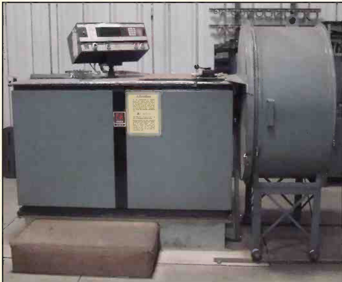
In house fan blade balancer capable of balancing blades from 12" to 72" diameter.
